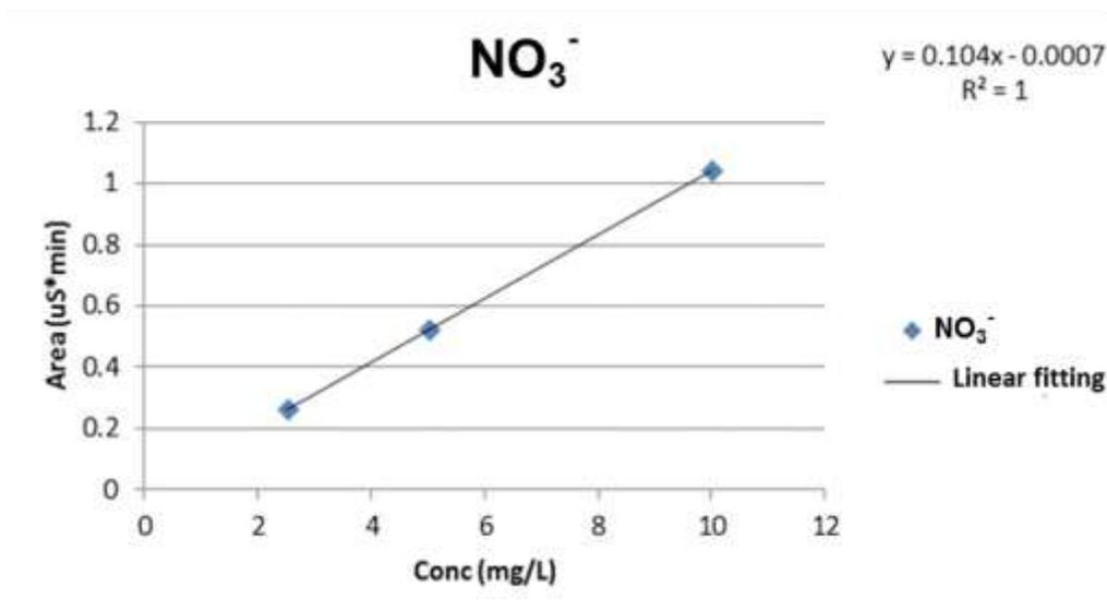
**Figure S19.** IC Calibration curve for nitrate anions.
