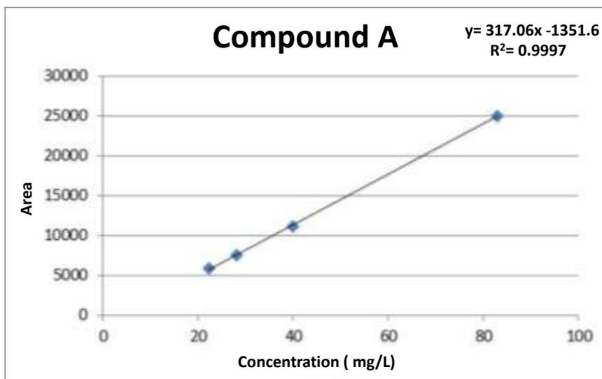
**Figure S3.** GC-MS Calibration curve for compound A.
