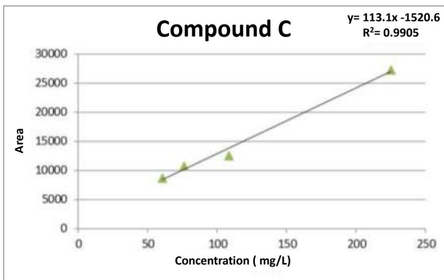
**Figure S5.** GC-MS Calibration curve for compound C.
