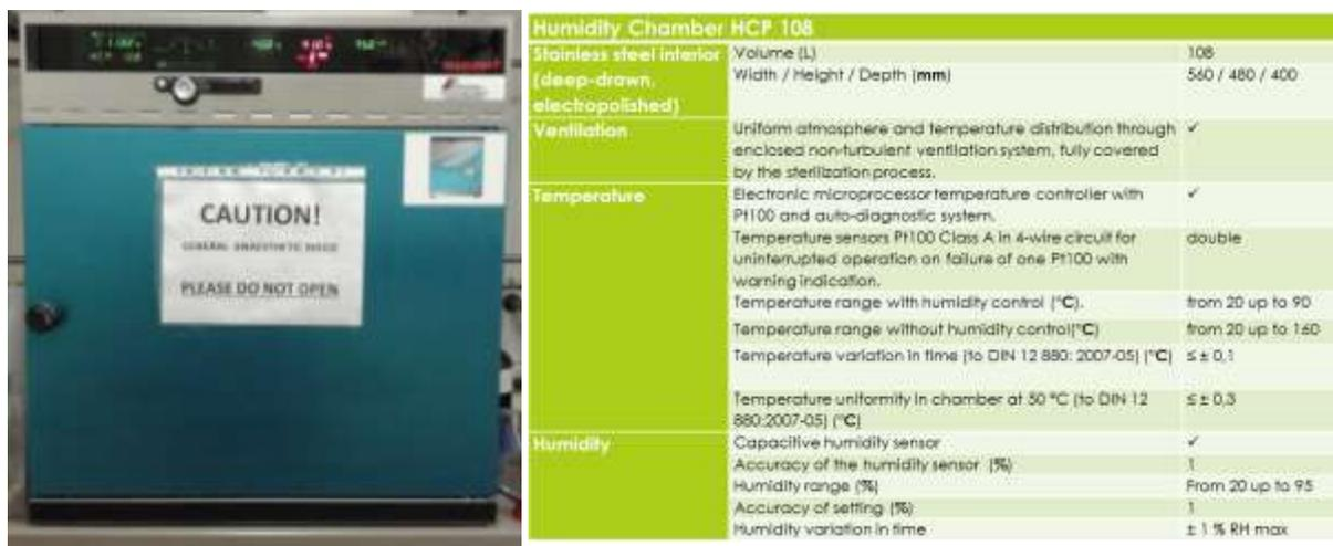
**Figure S2.** Memmert Humidity Chamber (HCP108) used for storage at 40 °C and 75% RH conditions (*aa*) and some technical characteristics of the chamber.
