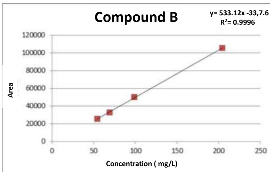
**Figure S4.** GC-MS Calibration curve for compound B.
