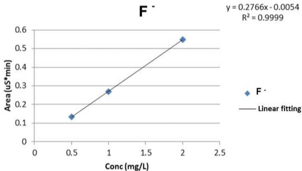
**Figure S17.** IC Calibration curve for fluoride anions.
