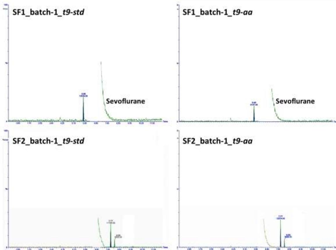
**Figure S8.** Top: GC-MS chromatograms of **SF1\_batch-1\_t9-std** (left) and **SF1\_batch-1\_t9-aa** (right); Bottom: GC-MS chromatograms of **SF2\_batch-1\_t9-std** (left) and **SF2\_batch-1\_t9-aa** (right).
