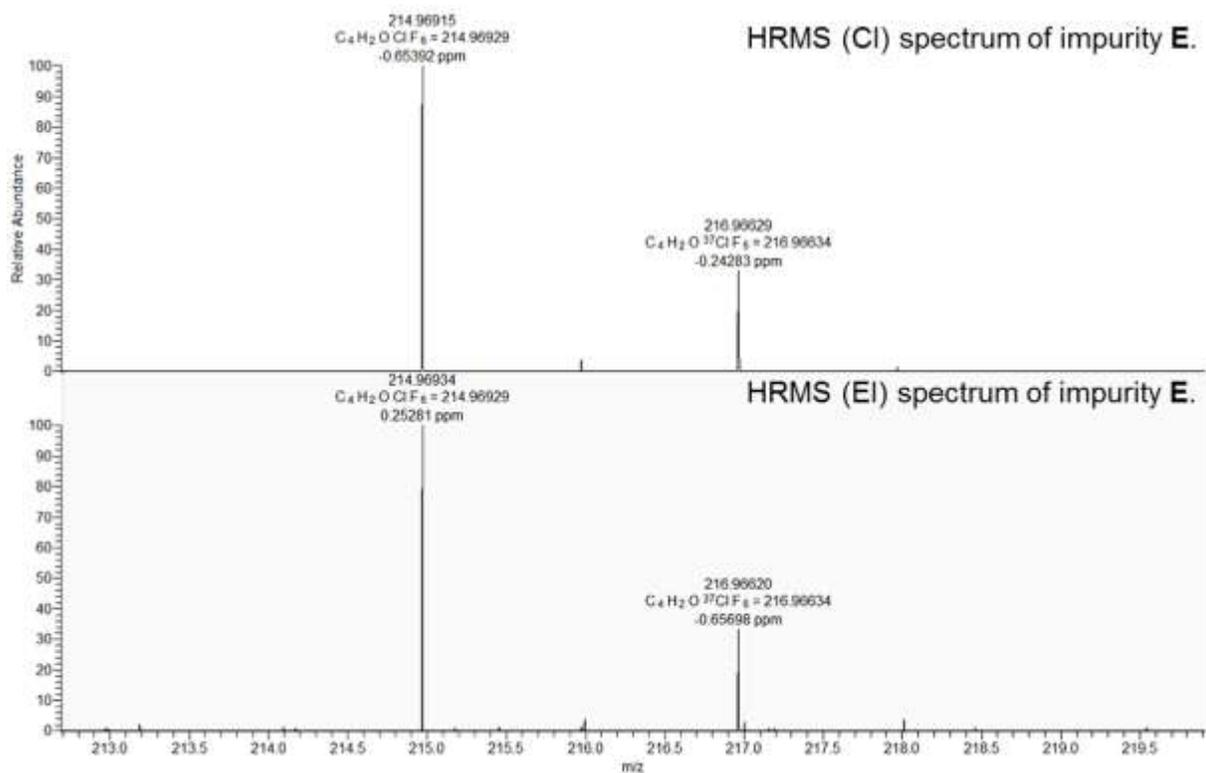
**Figure S15.** HRMS spectrum of impurity **E** showing molecular peaks after Chemical Ionization (CI, top) and after Electron Impact (EI, bottom).
