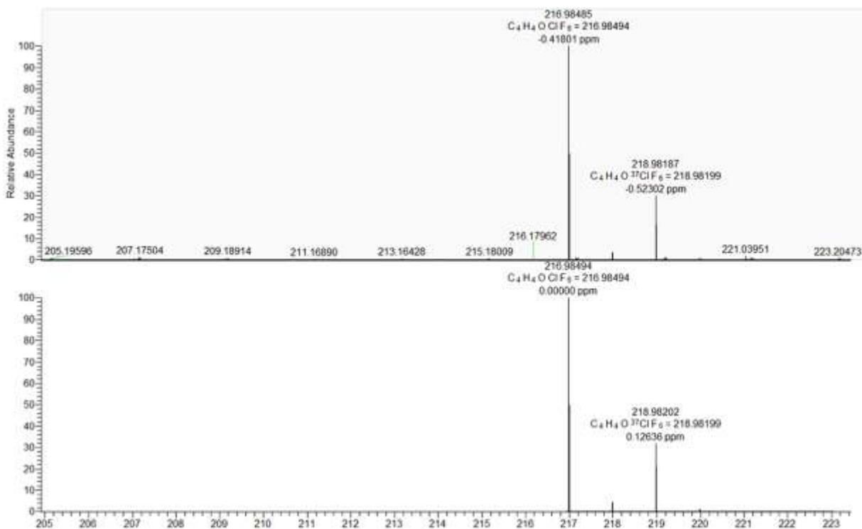
**Figure S14.** Top: HRMS spectrum of impurity **D** showing molecular peaks after Chemical ionization (CI); Bottom: Theoretical molecular formula and corresponding predicted HRMS peaks.
