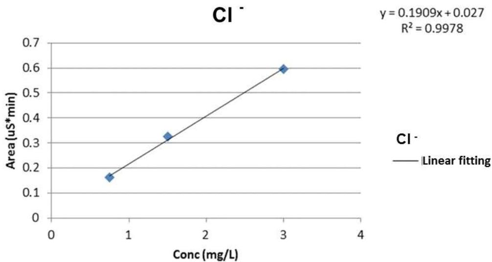
**Figure S18.** IC Calibration curve for chloride anions.
